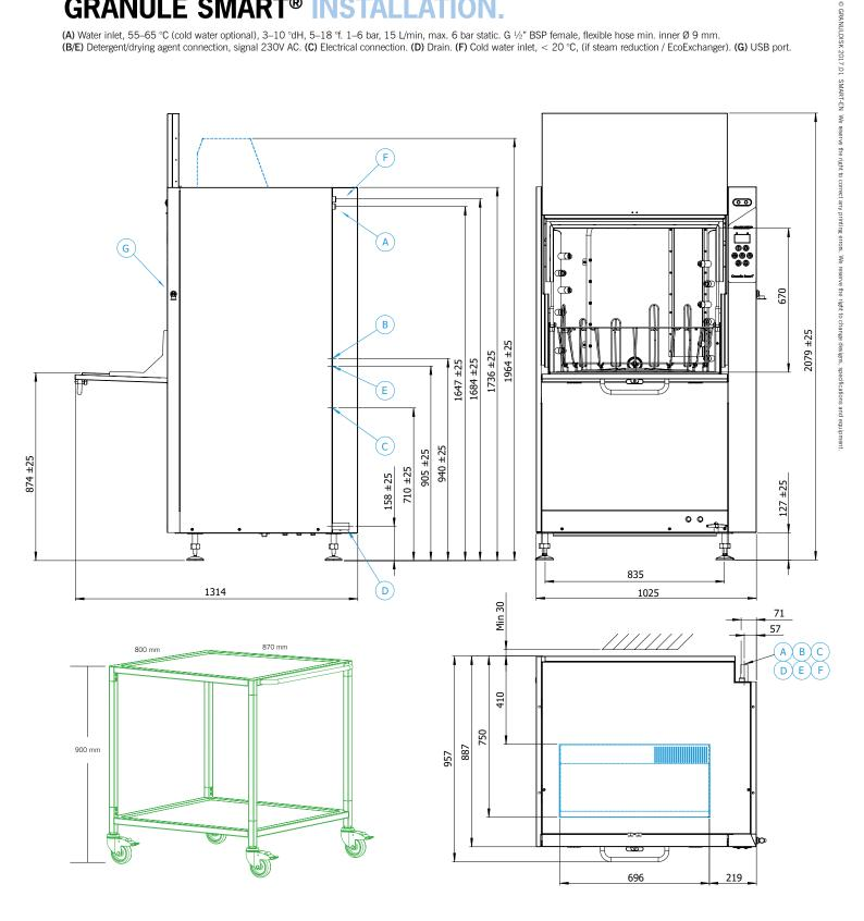
© EcoExchanger® unit (optional add-on). The EcoExchanger unit (heat recovery and steam reduction) must be connected to a cold water feed at all times.(F) Note: EcoExchanger is only available for cold water option machines (max power 32A, 16,5 kW) but on site, the machine can be connected to either a hot or a cold water feed. (A)
