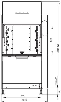
**A Water supply:** 3-10 °dH, 15 l/min, Temperature 50-65°C (cold water optional)
