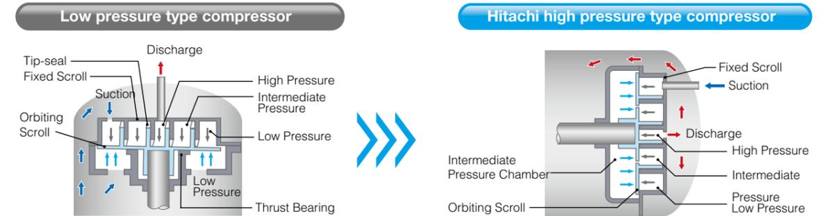
The end plate of the orbiting scroll is supported in the middle by the thrust bearing. Tilting the orbiting scroll creates a gap between the orbiting scroll and the fixed scroll which is covered by a tip-seal.
