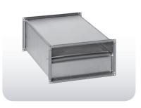
Silencers are produced using 30 mm rock wool insulation perfore sheet on the inside, aluzinc sheet metal on the outside.
